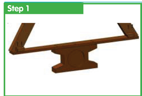
Ground Anchor Type 3 for models SG 180/200/FG 180/200
