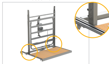
8.2.3 Bed end and backrest section assembled
